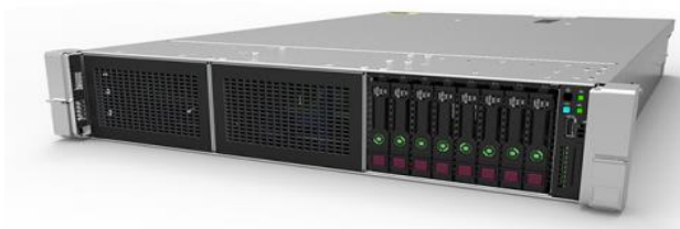
HP DL380 G9 2P E5-2620v3 2.40GHz 6-C 32GB (2x16GB) 2x500GB SATA 2x500W 2xRiser inclusief Rack-Kit (Refurbished)
